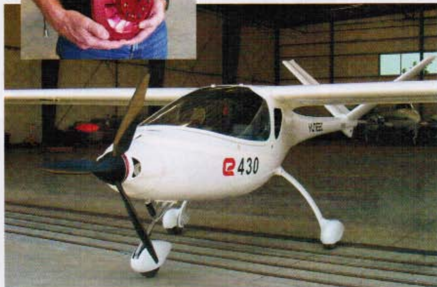
A 37-pound, 54-horsepower motor (left) powers the Yuneec, an electrically powered aircraft manufactured in China (below), which was flight tested in California recently.
