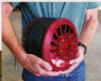
A 37-pound, 54-horsepower motor (left) powers the Yuneec, an electrically powered aircraft manufactured in China (below), which was flight tested in California recently.
